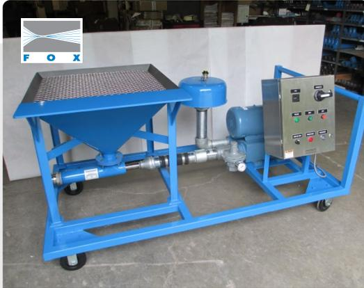
Fox can provide a blower + eductor conveying system, cart-or skid mounted to move wherever it is required. Note the small blower and eductor with no moving parts. Control panels can be provided with motor starters, interface and safety locks, and interface with destination level controls.
