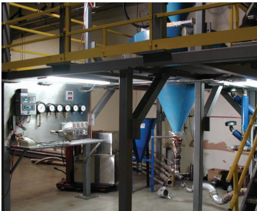
The test system can handle light- to high-density materials from micron size to 1-inch chunks at conveying pressures from 0.5 to 110 psi and conveying rates up to 12,000 lb/h.
