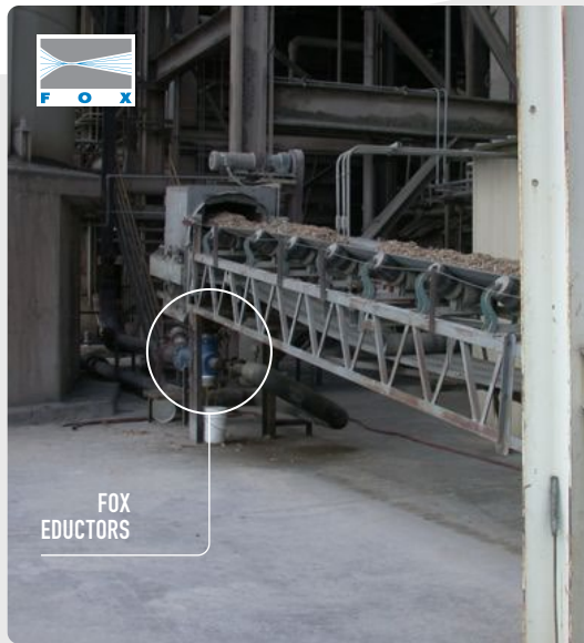
This Fox eductor, in blue, bolts up to the outlet of a long belt conveyor carrying wood chips.
