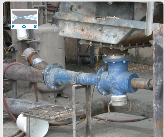
This Fox eductor, in blue, bolts up to the outlet of a long belt conveyor carrying wood chips.
