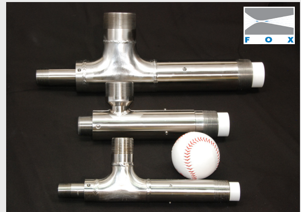
Three ceramic lined eductors with stainless steel housings. The ceramic liners are partially removed at the discharge to show how they are replaced in the field.
