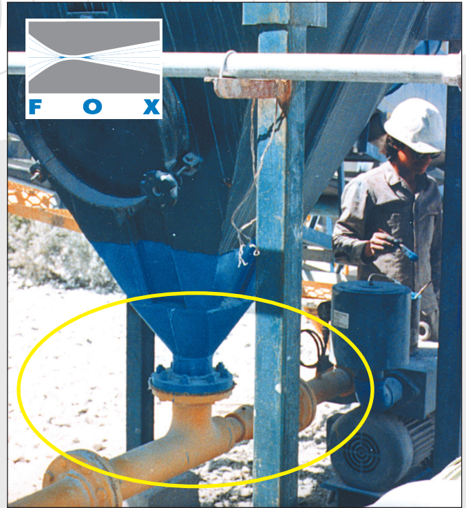
A carbon steel eductor conveys limestone dust at a mine in Mexico using air from a blower at 3 psig.
