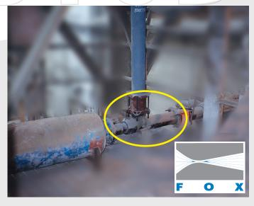
A ceramic lined Eductor conveys CAD at a cement plant.
